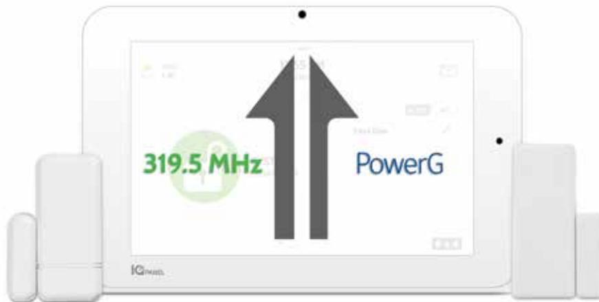
**Qolsys also offers encrypted sensors. The manufacturer's panels can take over older one-way sensors while enhancing the security installation by adding one- and two-way encrypted sensors to the original installation.**
